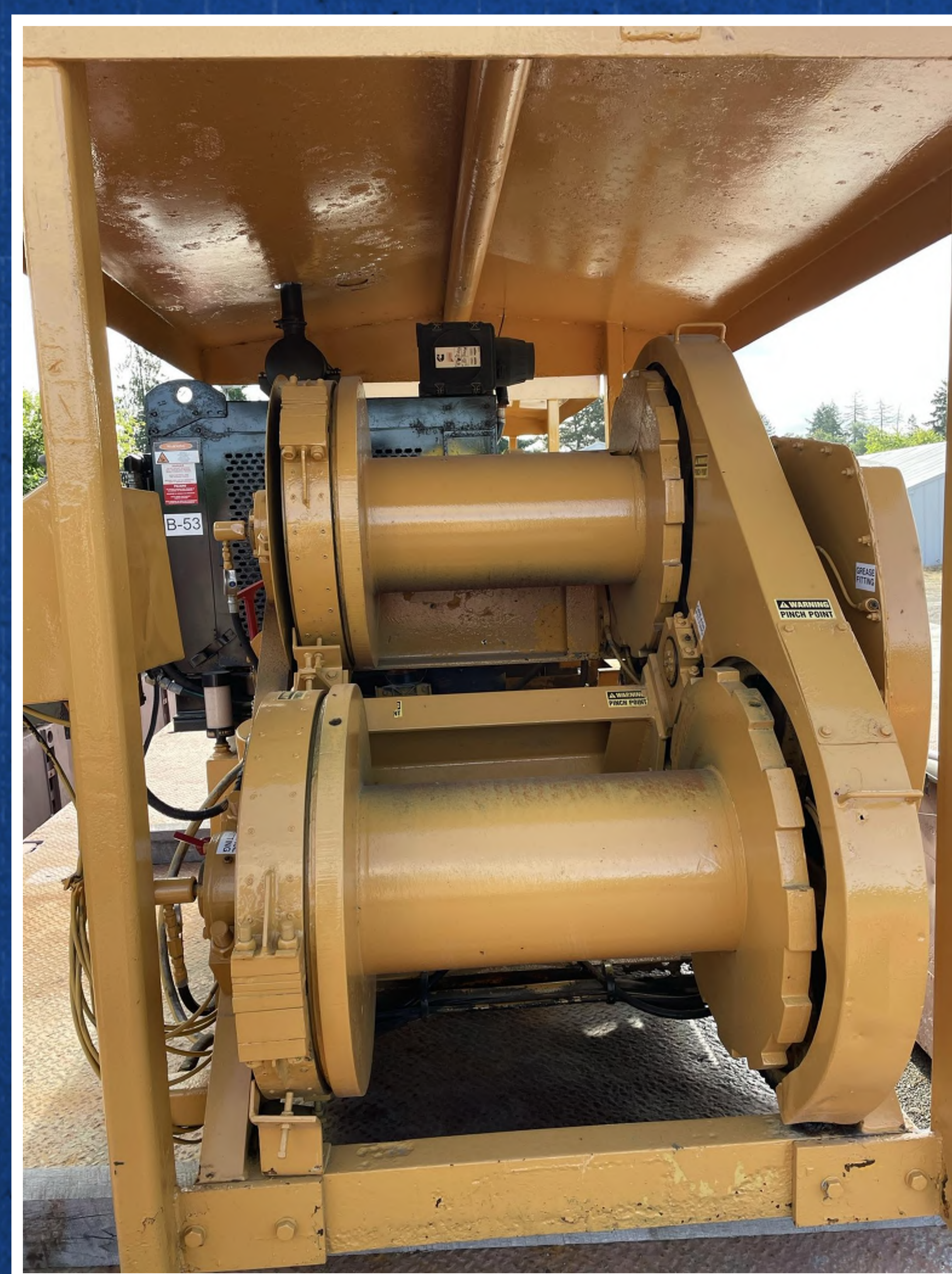
AMCON 150 HEAVY-DUTY AIR-CONTROLLED DOUBLE DRUM WATERFALL WINCH
